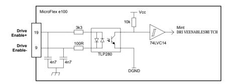
Figure 24 - Drive enable input circuit
